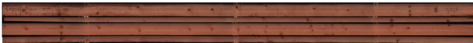
Figure 4: The four sides of a board. The dark, circular objects are the knots to be matched.
